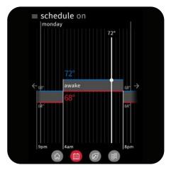
The **schedule screen** displays upcoming set point changes and scheduled times. Plus, it offers access to edit mode, where you can adjust the schedule using simple controls.
