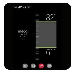
When you're away from home, you can help keep energy consumption down with away mode. The **away screen** displays energy-saving set points that can be invoked manually or automatically when the mobile app recognizes everyone is away.
